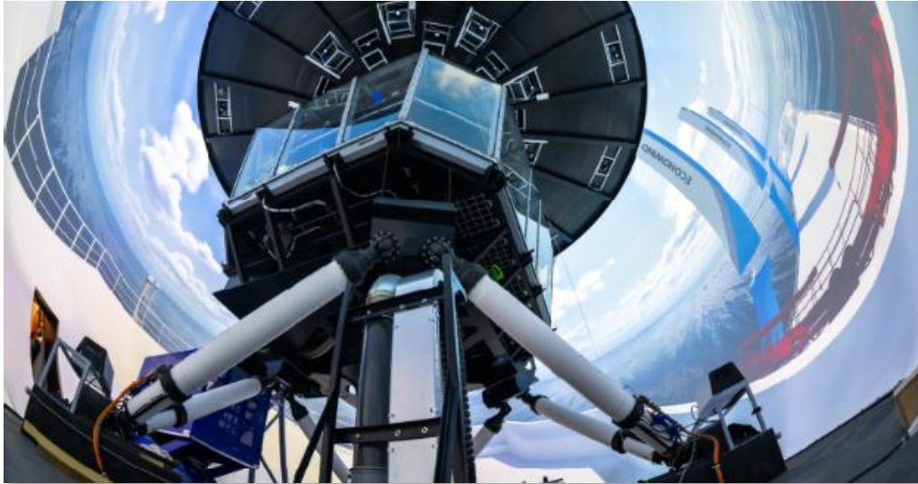
Large motions simulator with a moving platform
